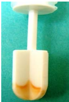
Figure VI. A close up photo image of a positive stick showing the narrow band formed due to shaking during incubation
